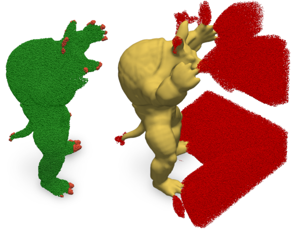
Figure 4: A neural DF f trained for a given shape S (yellow) using the method of [CB24]. Left: true positives (green) and false negatives (red) among 5M random test points; 796 points misclassified as outside. Right: points outside S where the distance is overestimated by f (red, 17% of 5M points). Notice how these volumetric overestimation regions originate from regions of false negatives.
